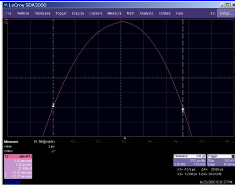
Figure 9. Total jitter curve. The vertical values of this curve represent the probability of a data transition occurring at a time represented by the horizontal axis. The horizontal center of the plot is 0 ps. The two markers are placed at the vertical level corresponding to a bit error rate of 10 e-12 and the horizontal distance between these two points is the total jitter at this bit error rate.
